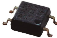
TS45S 1NA - Vmax=60V / Imax=100mA / SMD (4 pin SOP)
